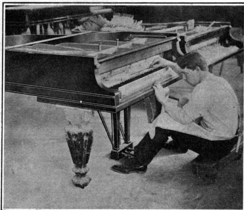
Regulating the Action of a Grand Piano.
