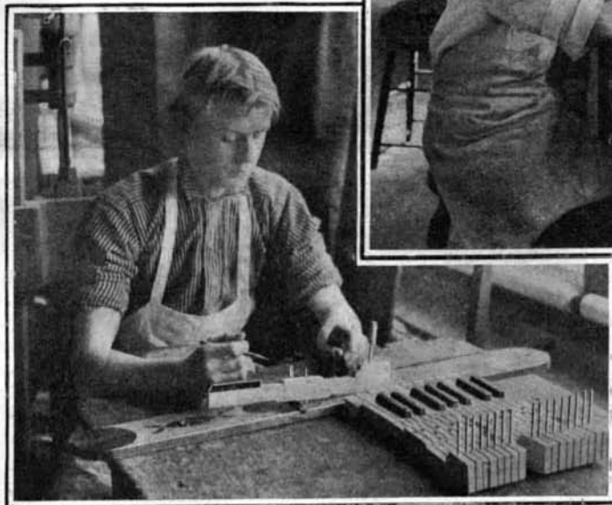
Balancing Each Key Individually.
