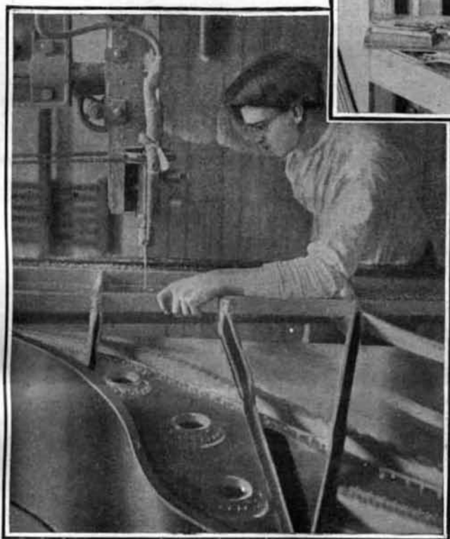
Drilling Holes for Tuning Pins in the Plate of a Grand Piano.
