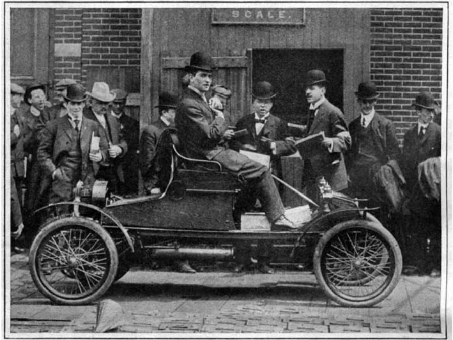
Light-weight Orient Buckboard Fitted With 4-Horse-Power Air-Cooled Motor and Friction Disk Transmission.
