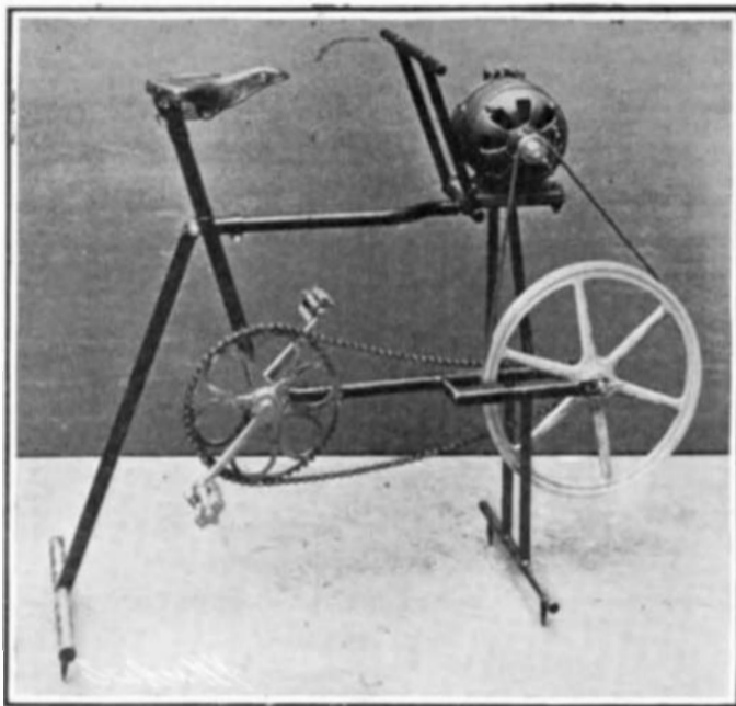
A BICYCLE GENERATING STATION USED BY THE GERMAN ARMY'S WIRELESS TELEGRAPH CORPS IN THE SOUTH AFRICAN CAMPAIGN.
