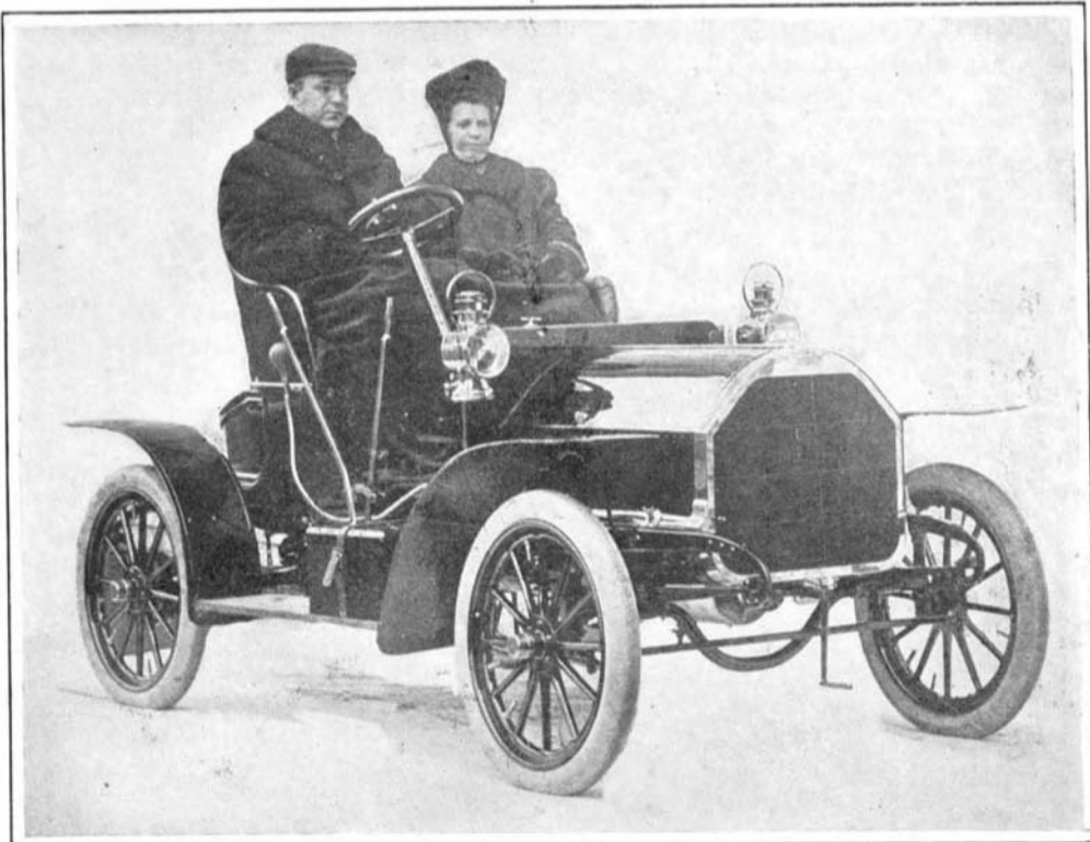
A 1,300-POUND RUNABOUT FITTED WITH A 16-HORSE-POWER, 4-CYLINDER, AIR-COOLED MOTOR.
