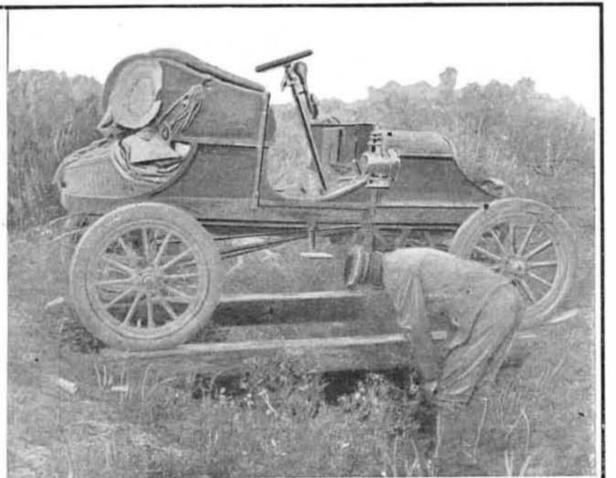
Temporary Bridge of Railroad Ties Near Bitter Creek, Wyoming.
