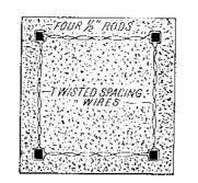
ment, it will be necessary to reinforce them (9966) H. N. asks: The ground is with steel roas. This can be done by means are used, it will be necessary to employ some device to keep the rods properly spaced as the I am told that the frost travels concrete is tamped into the mold. A simple method would be to use strong twisted wire spaced so as to come either end of post, and length.
