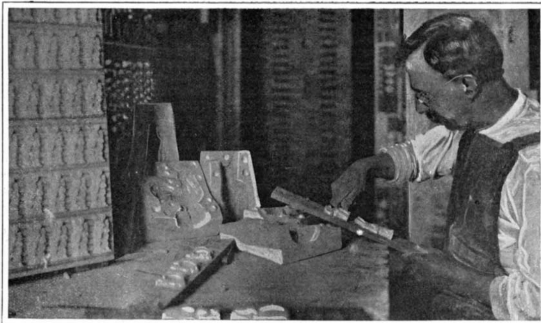
Carving Plaster Molds by Hand.
