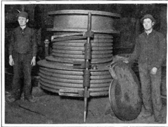
A Double-Grooved Drum and Cam Used in Striking Up the Mold.
