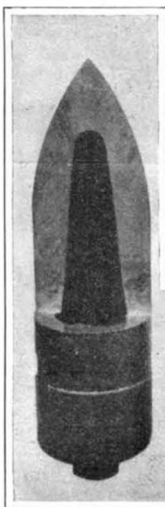
The 6-Inch Capped, Ribbed-Cavity Shell Which Was Loaded with Black Powder and Exploded Six Feet Behind a 6-Inch Kruppized Plate.
