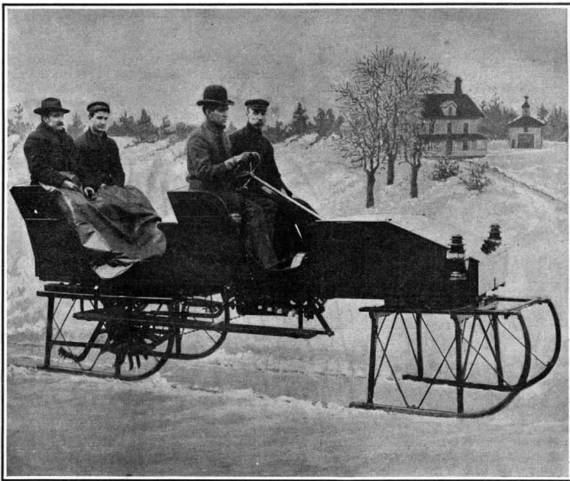
MOTOR SLEIGH SAID TO BE CAPABLE OF MAKING 35 MILES AN HOUR ON SNOW AND 90 MILES AN HOUR ON ICE.
