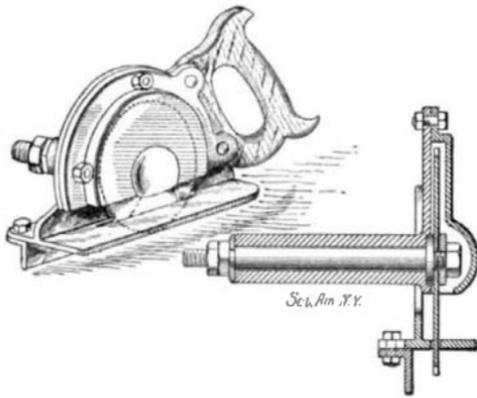
A PORTABLE ROTARY HAND-SAW.
