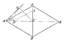
onals. Draw AG, making an angle of 45 deg. with AB, and let fall the perpendicular from C upon CG. With CG as a radius, describe the arc GH. CH is the semi-major axis of the ellipse. Draw HI parallel to AD, and IC is the semi-minor axis of the ellipse. From these the ellipse may be constructed.
