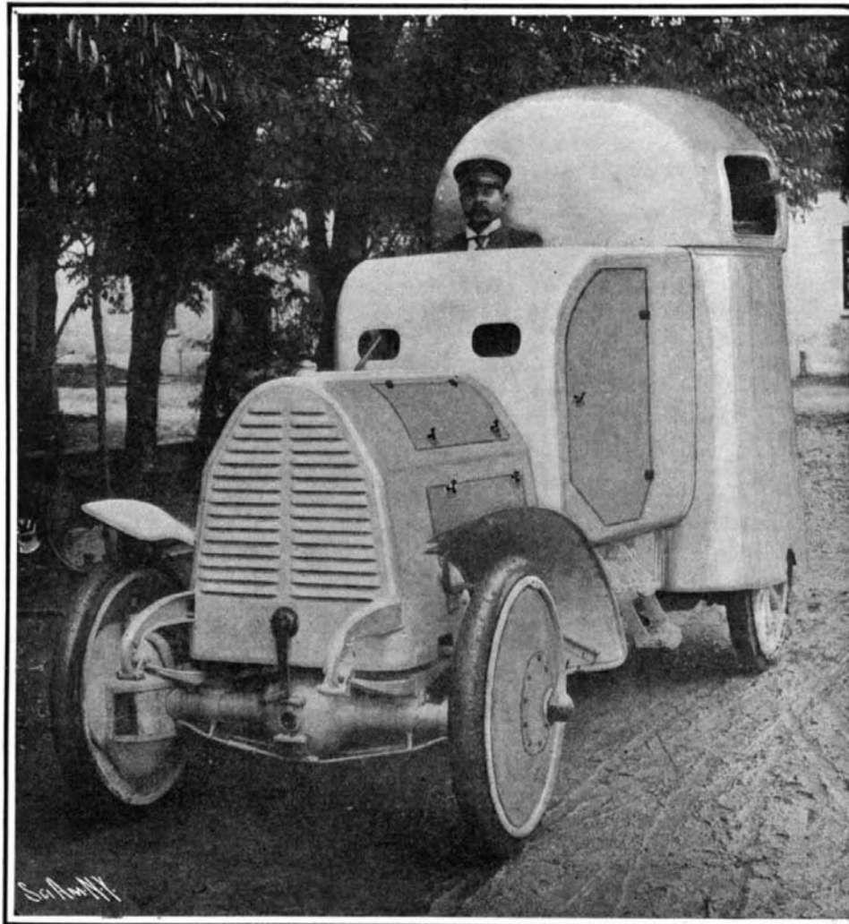
AN AUSTRIAN ARMORED WAR AUTOMOBILE. ALL FOUR WHEELS ARE DRIVERS.
