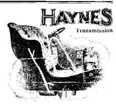
The transmission gear of the "Haynes" is sure, silent, and above all—simple. When the friction clutch that controls the master gears is released, and the clutch that locks the engine shaft engaged, the power is conveyed directly to the rear axle and all other gears in the transmission stand idle.
