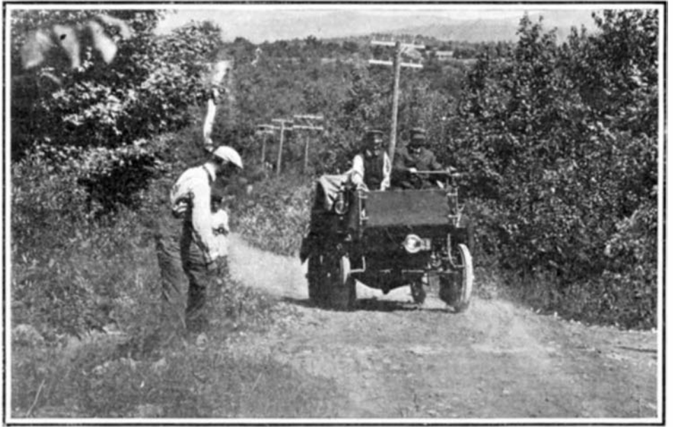
Knox 16-Horse-Power Truck Climbing a Grade of 23 Per Cent on Morey Hill.
