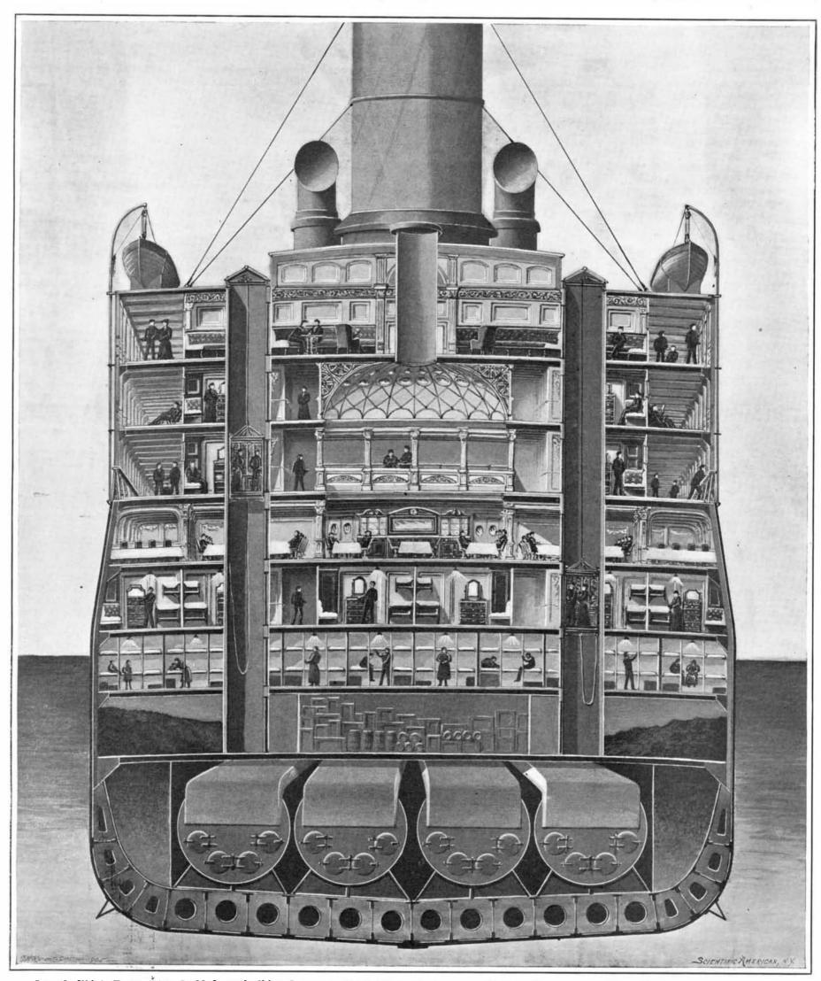
Length, 800 feet. Beam, 85 feet. Molded Depth, 60 feet. Maximum Draft, 36 feet. Displacement, 43,000 tons. Horse-power of Four Turbines, 75,000. Speed, 25 knots. These Are the First Transatlantic Liners to Adopt Passenger Elevators. Because of the Great Size of the Ships, the Average Stateroom Will Be 50 Per Cent Larger Than in the Existing Fast Passenger Steamers.
