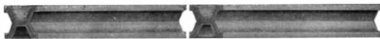
British Iridio-Platinum Yard Standard Showing Cross-Section. The Bar is in the Position it Occupies in the Comparator.
