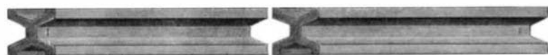
The Standard Turned on Its Side and Showing the Two Defining Lines (Magnified) on the Neutral Surface of the Bar.
