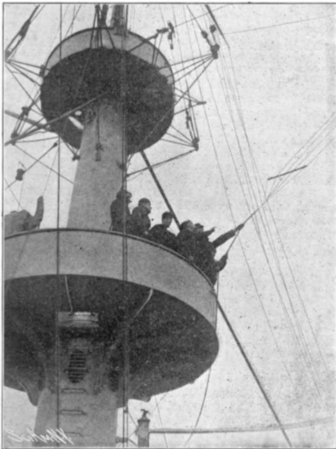
Class Observing Aerial Wires for Receiving and Sending on a Battleship.
