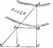
the near bank of the river, as B. Measure off any convenient distance—say one or two hundred feet—from B to the point C, which shall be in the line AB. Select a third tree or stake, as D, and complete on the ground the parallelogram BCED. Then find the point F on the ground which is in line with EC and also in line with DA, and measure the distance from E to F. Then AB will equal BD multiplied by BC divided by EF.
