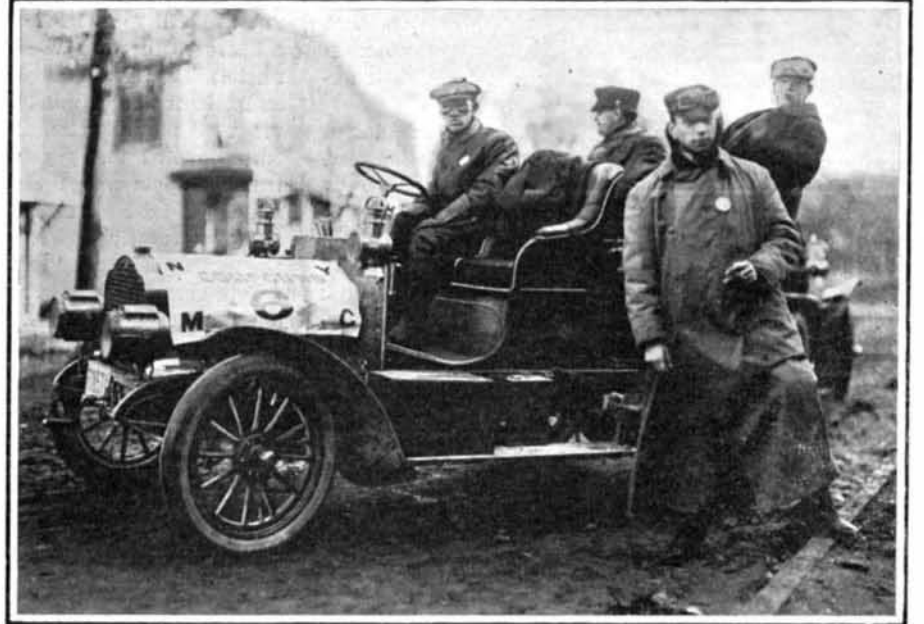
The 15-Horse-Power Compound Car Which Was Third. This car has two 4 \times 4 high-pressure cylinders and a third 7 \times 4 low-pressure cylinder between them.
