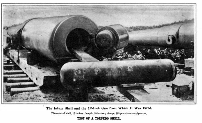
deterrent. Each of the separate chambers in the cell is provided with a screw plug opening through which the high explosive can be poured into the shell; the plugs being afterward screwed tightly
