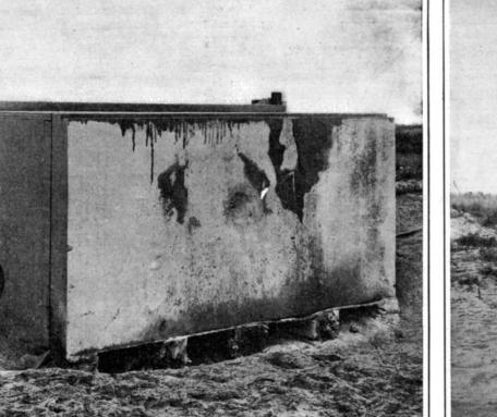
11½-Inch Plate After Being Struck by Isham Torpedo Shell-Practically Intact.
