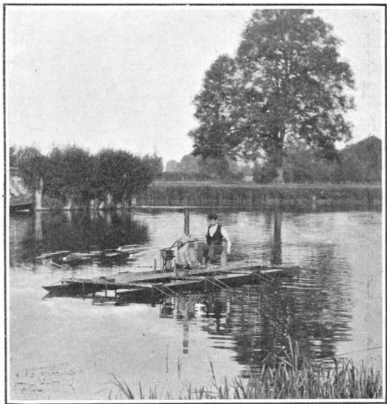
Lambert's Steam Glider, Model of 1897. Made 20 Miles per Hour.
