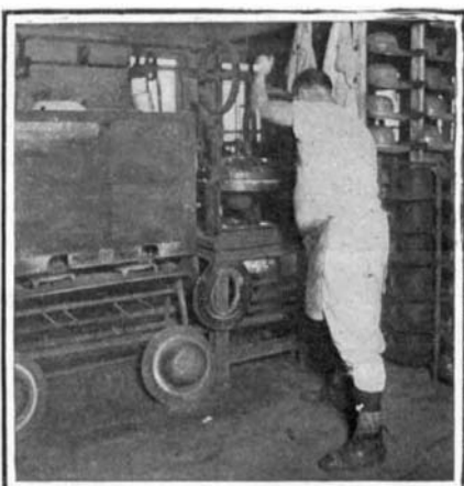
Finishing the Crown in the Hydraulic Press Which Gives It the Final Shape.
