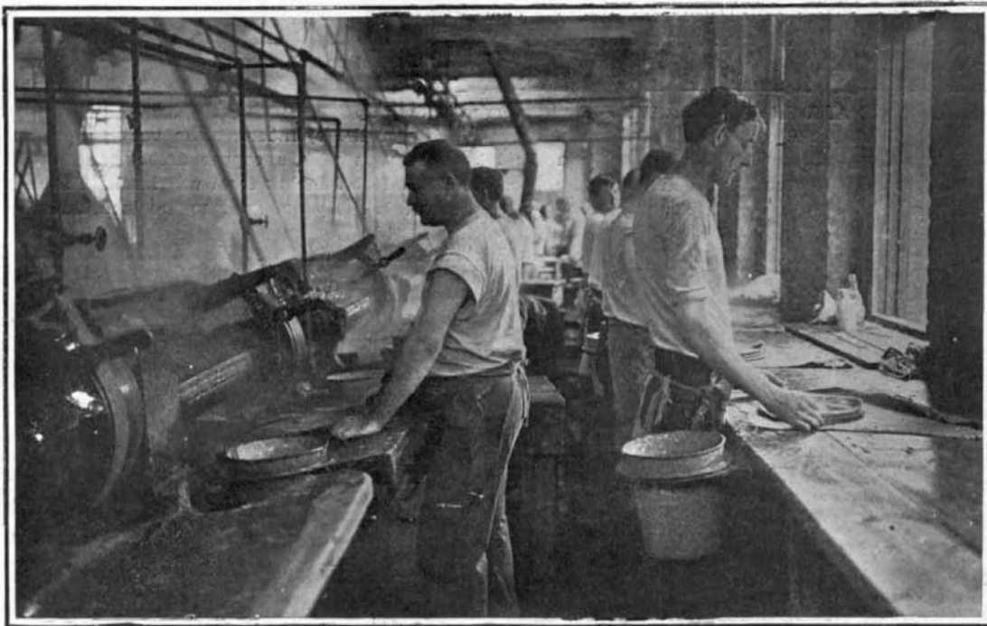
First-sizing. In This Operation the Felted Body Receives Its First Shrinking.
