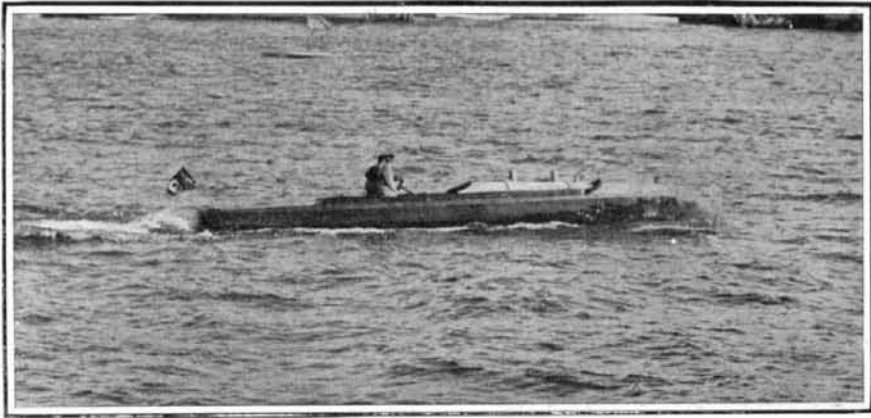
The 150-Horse-Power "Dixie," Which Won the International Trophy and, in One Circuit of the 10-Nautical-Mile Course, Developed a Speed of 24.19 Knots (27.82 Statute Miles an Hour).
