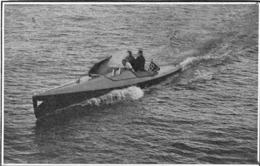
The 75-Horse-Power "XPDNC," Which Won the National Trophy and Maintained a Speed of 21.41 Knots (24.68 Statute Miles an Hour) Over a 30-Nautical-Mile Course.
