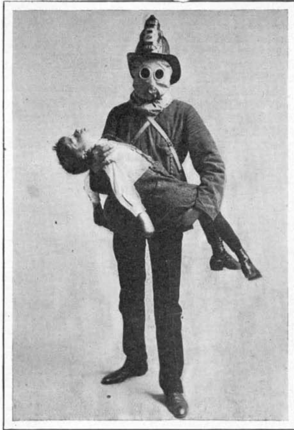
A Hood Lined with Oiled Silk Covers the Head of the Fireman.
