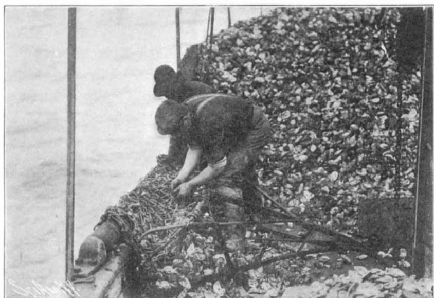
Deck of a Dredge Boat, Showing Crew Repairing a Break in the Dredge.
