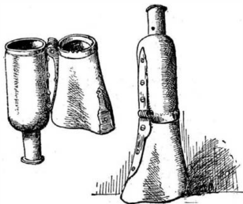
A "tinker's" Mortar from Grosse's Military Antiquities, 1801. "An uncommon engine supposed to be a tinker's mortar, which being fixed in a stick was used for throwing grenades."
