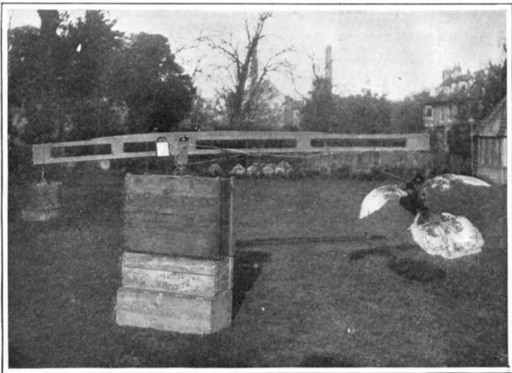
Apparatus for Demonstrating the Lifting and Propulsive Effect of a Bird's Wings.
