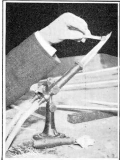
Heating the End Before Blowing.
