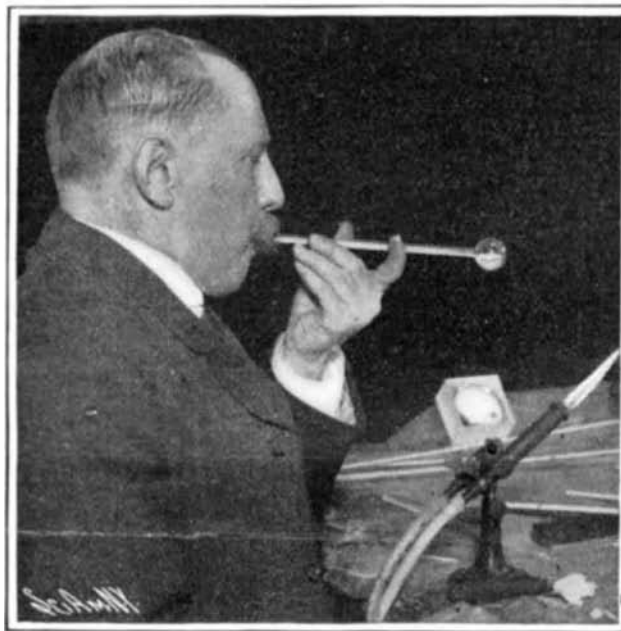
After the End Has Been Heated in the Blowpipe the Bulb is Blown.
