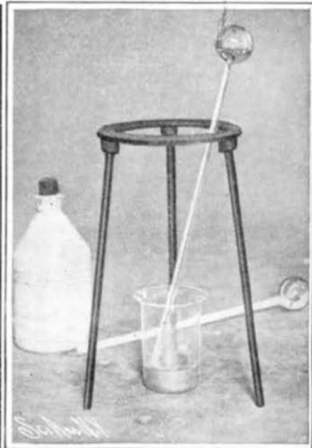
Immersing the Tube in Mercury so That the Metal Rushes Up to Fill the Vacuum.
