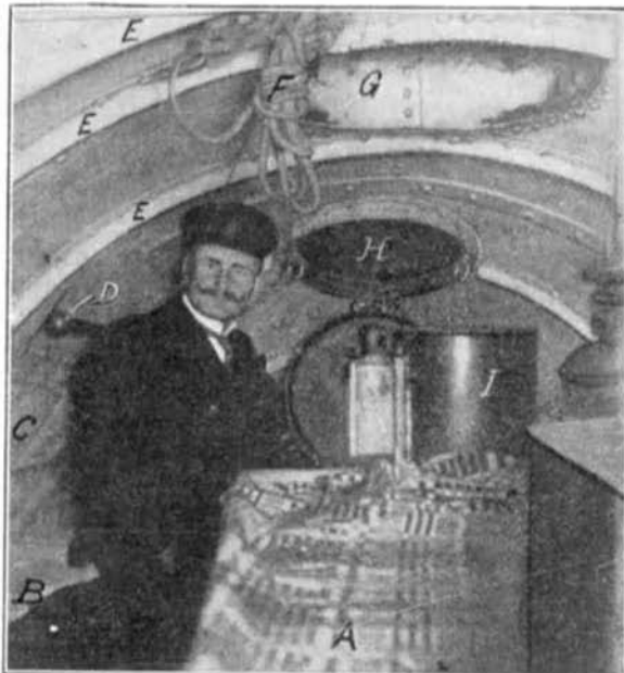
A , table; B , seats or berths; C , cork pads for protection; D , tiller; E , frames (steel angles); F , main sheet led through deck; H , watertight hatchway.
