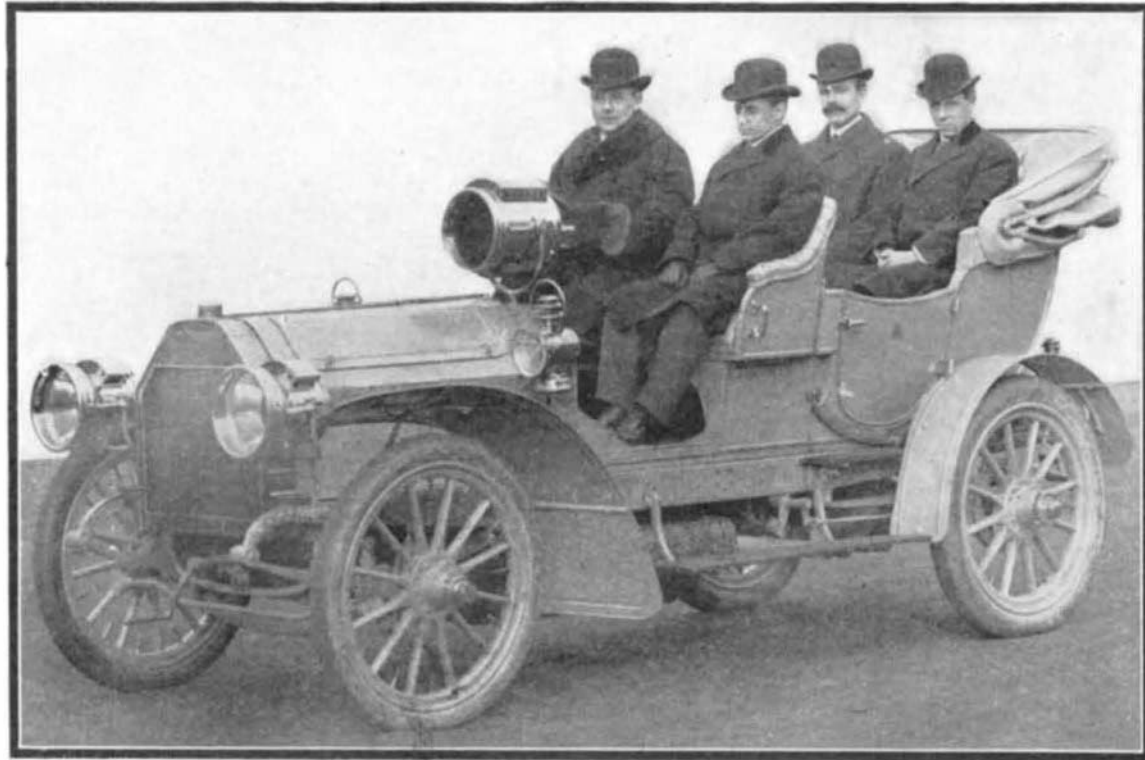
The Peerless 60-Horse-Power Side Entrance Tonneau Fitted with Bevel Gear Drive.
