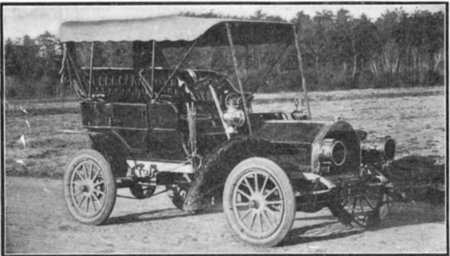
The Stevens-Duryea 20-Horse-Power Side Entrance Tonneau Fitted with 4-Cylinder Vertical Engine.
