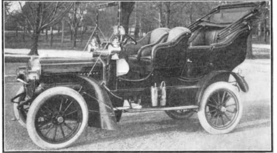
Thomas 4-Cylinder 40-Horse-Power Side Entrance Tonneau Fitted with Chain Drive.
