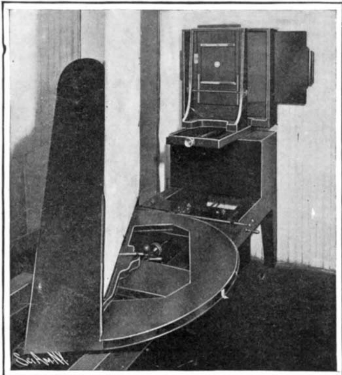
Enlarging Apparatus; 11-Foot Bed. Easel is Turned About to Show Its Face. Lens Can be Moved by Means of Guide Rod from Any Position Along the Bed.
