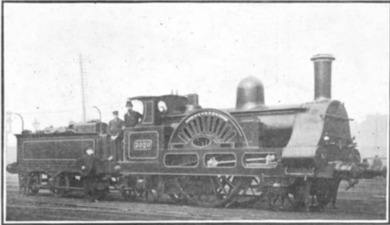
Fig. 2.—Express Engine "Cornwall" as It Is Running To-day. Largest Driving Wheels in the World.
