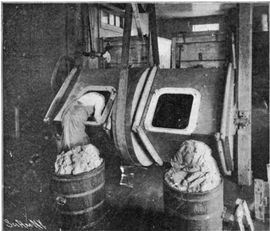
Taking the Butter from the Steam Churn, Which Holds 350 Gallons. The Tubs of Butter Were Churned in One Hour.
