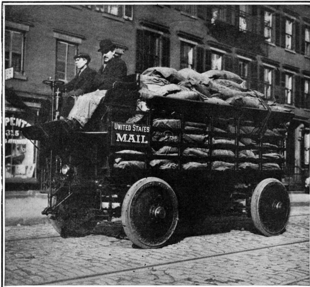
ELECTRIC TRUCK WITH MOTORS IN WHEELS TRANSPORTING UNITED STATES MAIL.
