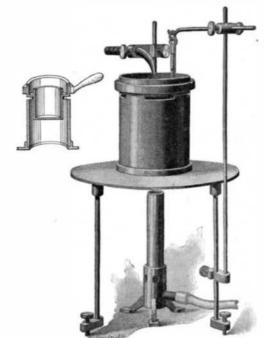
APPARATUS FOR TESTING FLASHING POINTS OF OILS.
