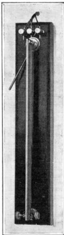
Thermostat for Regulating Temperature of Clockroom.
