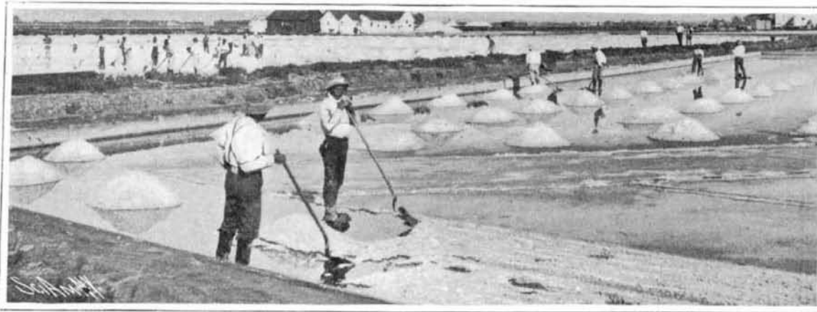
Scraping Salt From Hollow Settling Basin.
