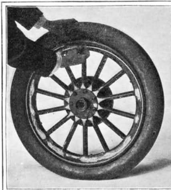
Fig. 2.—Removing the Small Locking Ring.
