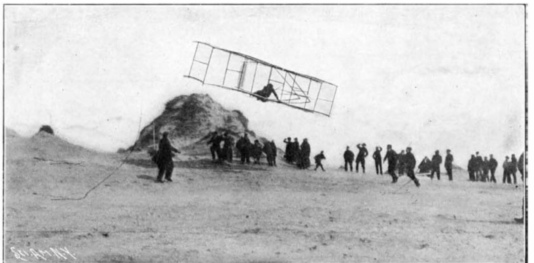
A Flight That Ended in a Fall Because the Wind's Direction Had Not Been Considered.
