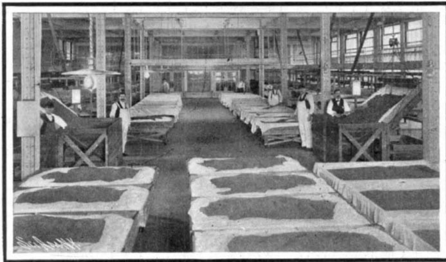
Drying the Thoroughly Cleaned and Cooked Grain Before Shredding.
