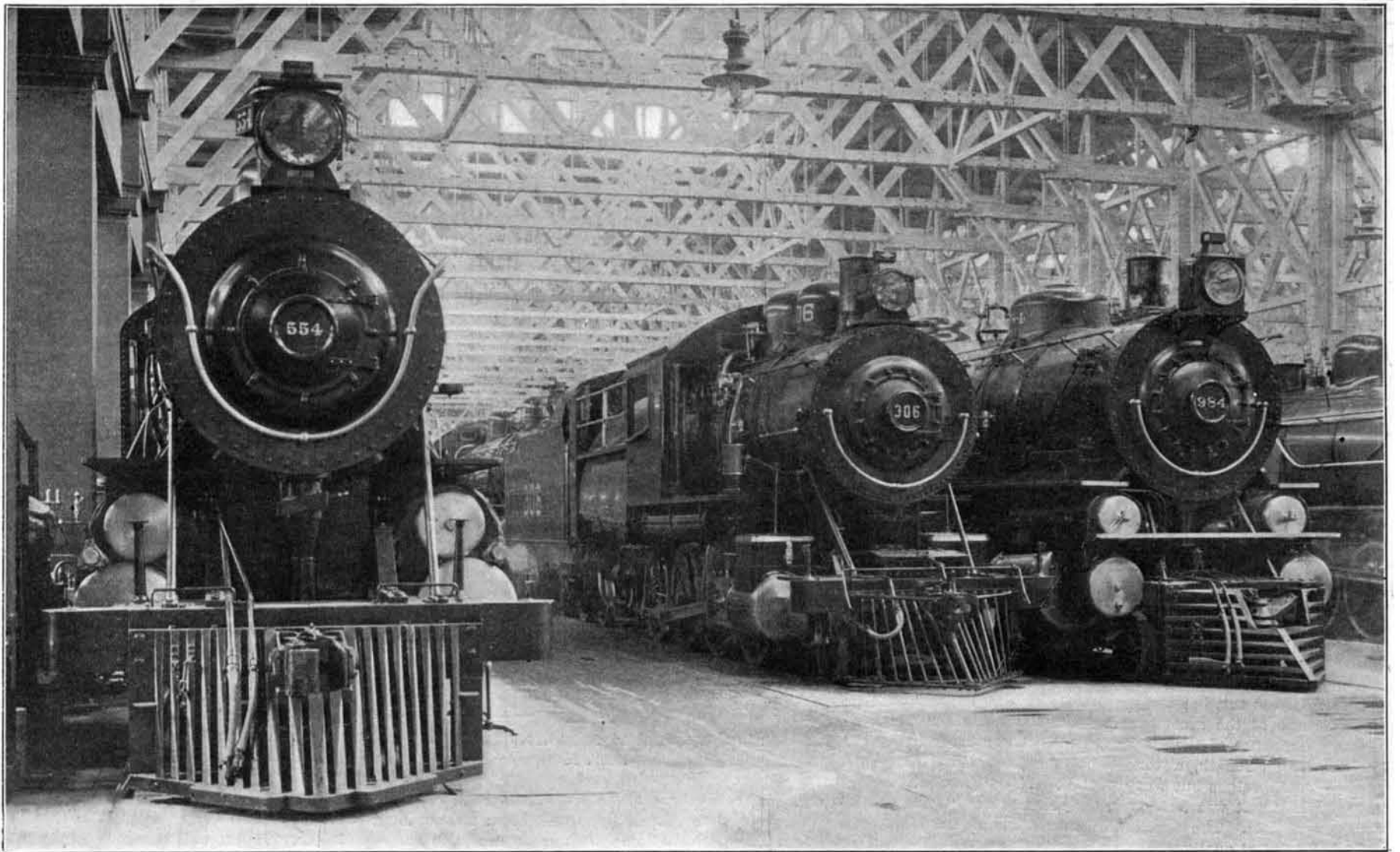
Cylinders, 20 x 28 inches. Heating surface, 2,655 square feet. Weight, 183,700 pounds. Atlantic Type Passenger Engine.
