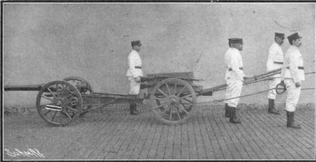
Three-Inch Rapid-Fire Gun with Limber Attached, Showing Method of Hauling by Gun Detachment.
