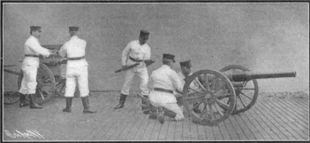
Japanese 3-Inch Naval Field Gun in Action. Limber Detached and Ammunition Being Transferred to Gun.
