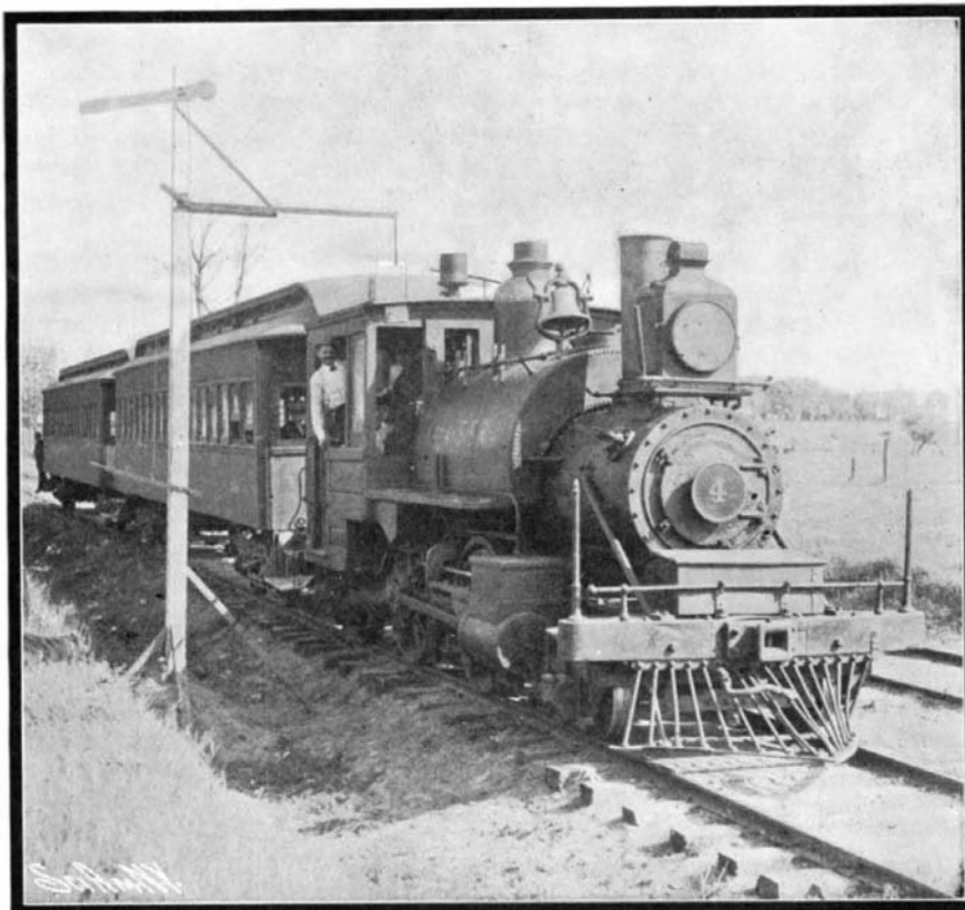
BLOCK SIGNAL DIRECTLY CONTROLLING THE THROTTLE OF A LOCOMOTIVE.
