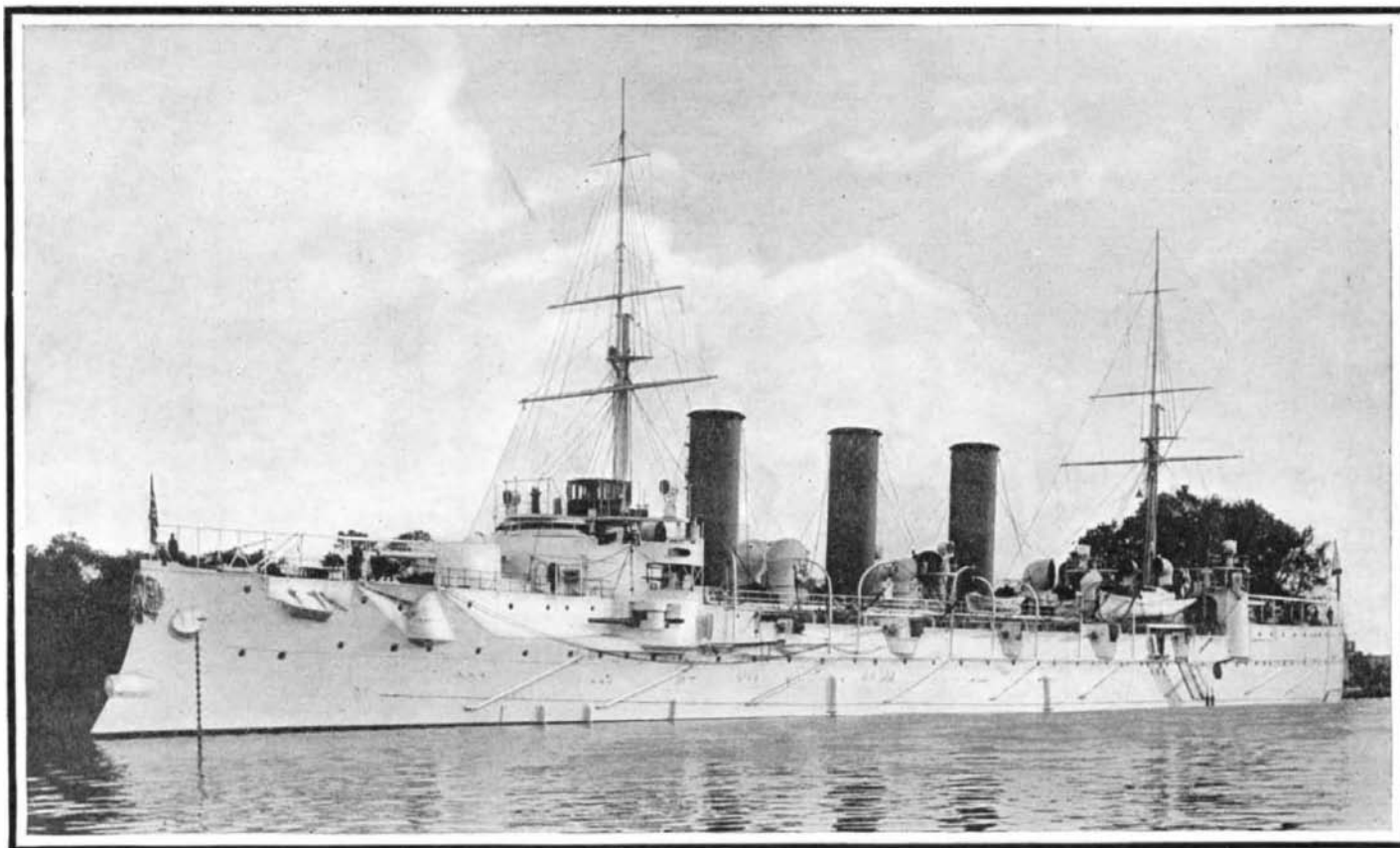
Displacement, 6,500 tons. Speed, 23.45 knots. Guns: 12 6-in., 12 3-in., 9 small guns. Armor: deck 2 in., casemates, 4 in. Torpedo Tubes, 6.
