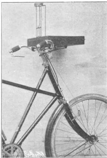
Fig. 1.—THE CYCLOGRAPH ON A BICYCLE.
