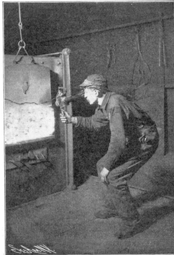
Measuring the Temperature of a Hardening Furnace.
