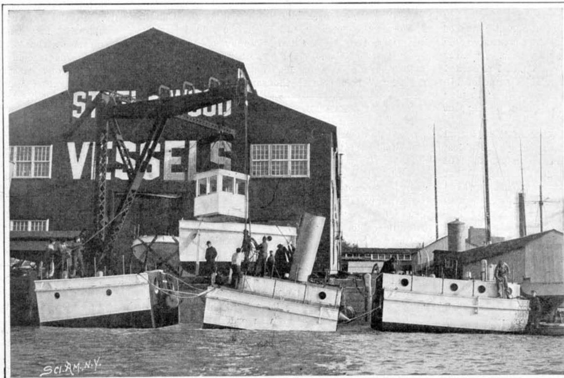
THE "PONTONIER" Afloat in the detached condition. Each section is capable of floating independently.
